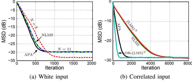
Fig. 1. APA, NLMS,  $\{\text{LMS}\}^N$ , and DR- $\{\text{LMS}\}^N$  ( $M = 100$ ,  $K = 10$ ,  $\eta_n = 1$ ,  $\mu_n = \mu$ ). (a) APA:  $\mu = 0.3$ ; NLMS:  $\mu = 1$ ; and  $\{\text{LMS}\}^N$ :  $\mu = 3 \cdot 10^{-3}$ ,  $N = 20$ ; (b) APA:  $\mu = 0.015$ ; NLMS:  $\mu = 0.9$ ;  $\{\text{LMS}\}^N$ :  $\mu = 1.5 \cdot 10^{-3}$ ,  $N = 30$ ; and DR- $\{\text{LMS}\}^N$ :  $\mu = 2 \cdot 10^{-3}$ ,  $N = 15$ .
