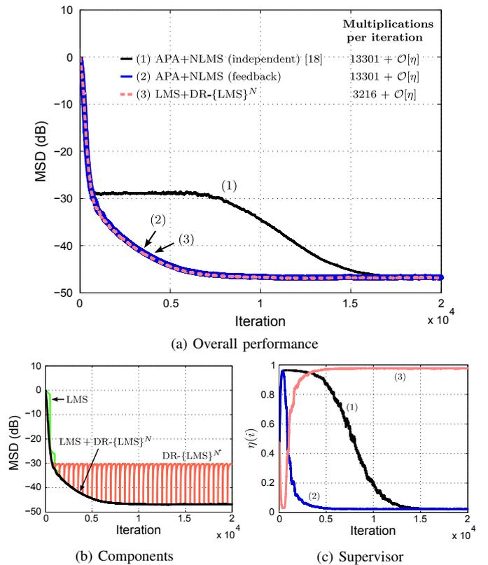
Fig. 5. **Parallel-incremental combination (correlated input)** ( $M = 100$ ,  $K = 10$ ,  $\eta_n = 1$ , and  $\mu_n = \mu$ ). **APA+NLMS**:  $\mu_{\text{APA}} = 1$ ,  $\mu_{\text{NLMS}} = 0.04$ ,  $\mu_a = 0.8$ ,  $\beta = 0.95$ ,  $\epsilon = 10^{-4}$ ,  $L = 400$ ; **LMS+DR- $\{LMS\}^N$** :  $\mu_{\text{LMS}} = 4 \cdot 10^{-4}$ ,  $\mu_{\text{DR- $\{LMS\}^N}}$  =  $2 \cdot 10^{-3}$ ,  $N = 15$ ,  $\mu_a = 0.7$ ,  $\beta = 0.95$ ,  $\epsilon = 10^{-4}$ ,  $L = 500$ .$
