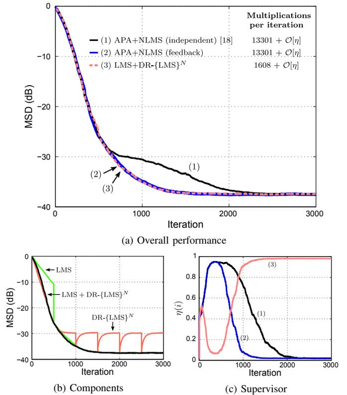
Fig. 4. **Parallel-incremental combination (white input)** ( $M = 100$ ,  $K = 10$ ,  $\eta_n = 1$ , and  $\mu_n = \mu$ ). **APA+NLMS**:  $\mu_{\text{APA}} = 0.3$ ,  $\mu_{\text{NLMS}} = 0.3$ ,  $\mu_a = 0.8$ ,  $\beta = 0.95$ ,  $\epsilon = 10^{-4}$ ,  $L = 400$ ; **LMS+DR- $\{LMS\}^N$** :  $\mu_{\text{LMS}} = 3 \cdot 10^{-3}$ ,  $\mu_{\text{DR- $\{LMS\}^N}}$  =  $6 \cdot 10^{-3}$ ,  $N = 7$ ,  $\mu_a = 0.7$ ,  $\beta = 0.95$ ,  $\epsilon = 10^{-4}$ ,  $L = 400$ .$
